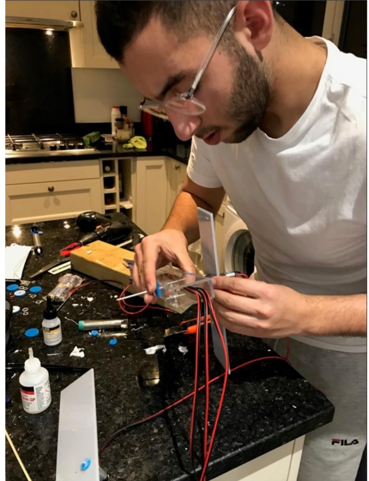
Gluing the parts and assembling the motors and gears to the body
