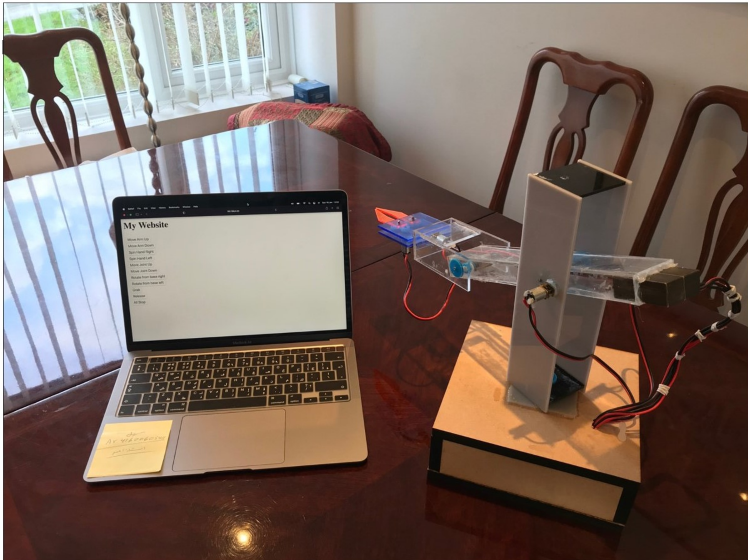
Working prototype robot with web server
