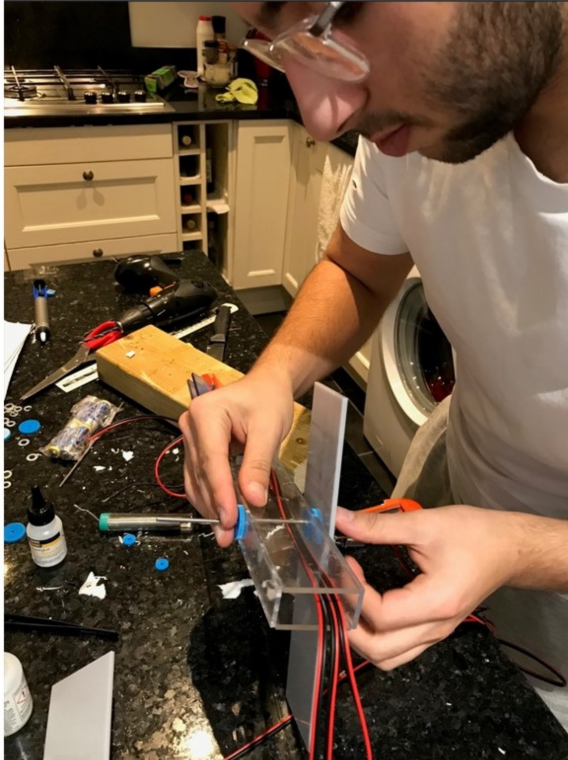
Gluing the parts and assembling the motors and gears to the body
